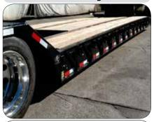
With a standard deck height of 24", Globe Trailers have lower overall height, which allows taller loads to be hauled.
