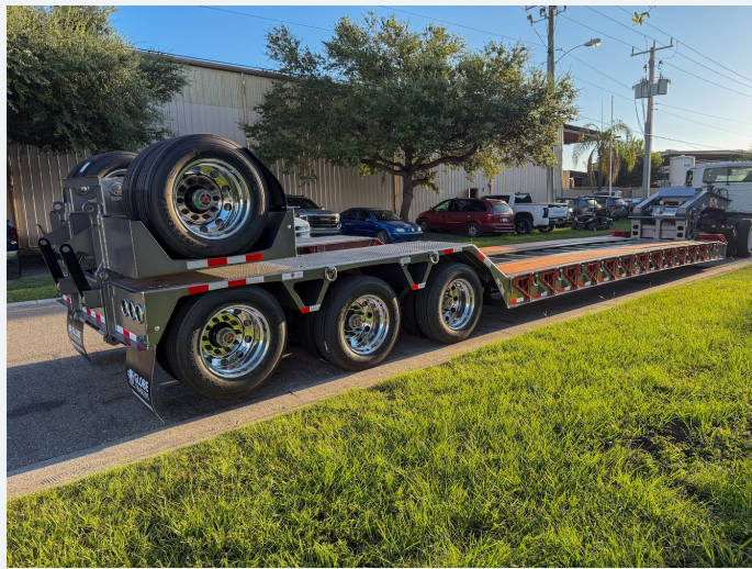
Hydraulic flip axle folds up for transport
