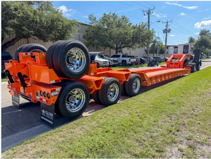
Hydraulic flip axle folds up for transport
