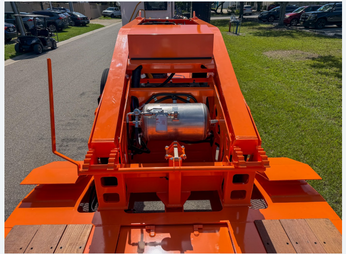
Gooseneck-mounted hydraulic power unit
