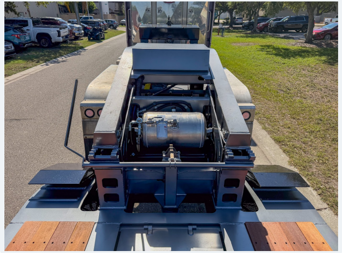
Gooseneck-mounted hydraulic power unit
