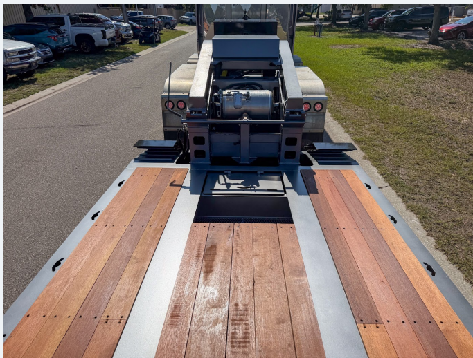
Apitong hardwood deck with recessed wells
