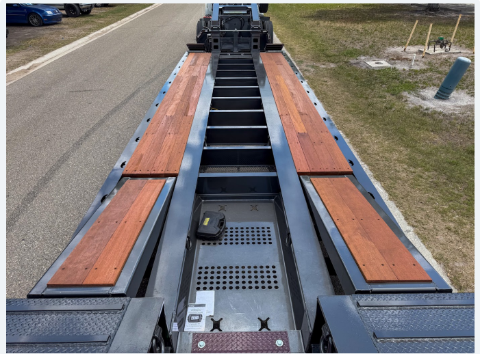
Apitong hardwood deck with recessed wells
