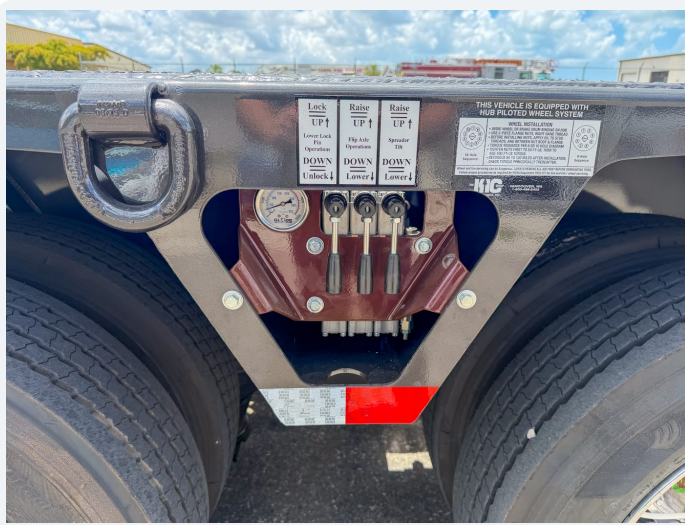
Clearly labeled air and hydraulic controls
