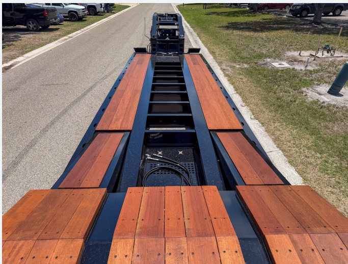
Apitong hardwood deck with recessed wells
