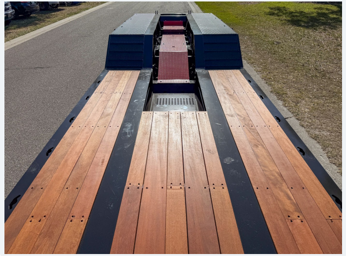
Apitong hardwood deck with recessed wells
