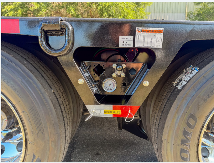
Clearly labeled air and hydraulic controls
