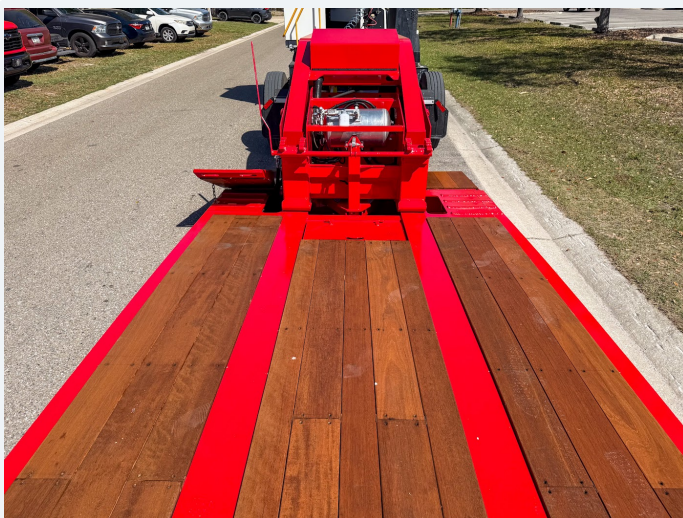
Apitong hardwood deck with recessed wells
