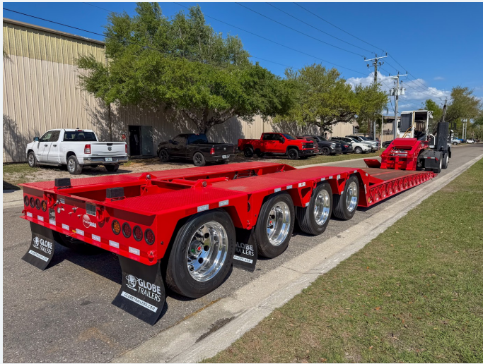
Hydraulic flip axle folds up for transport
