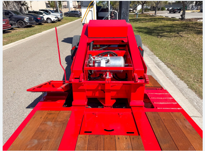
Gooseneck-mounted hydraulic power unit
