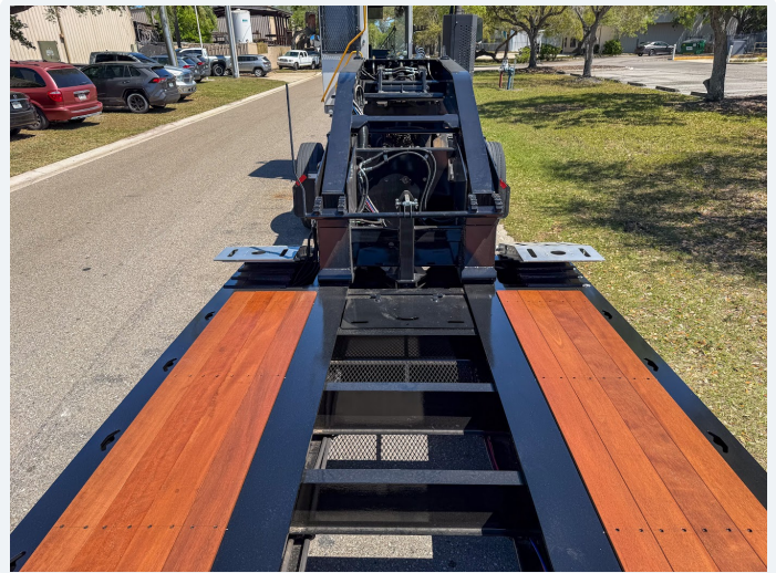
Apitong hardwood deck with recessed wells
