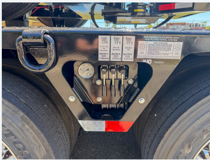
Clearly labeled air and hydraulic controls
