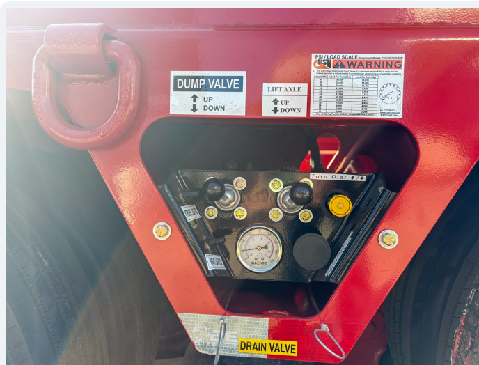
Clearly labeled air and hydraulic controls
