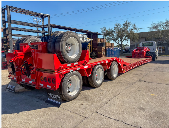
Hydraulic flip axle folds up for transport
