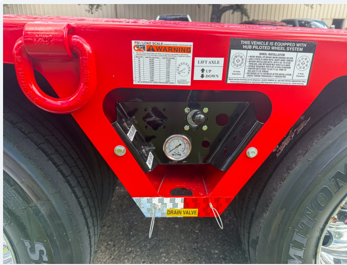
Clearly labeled air and hydraulic controls
