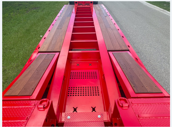
Apitong hardwood deck with recessed wells
