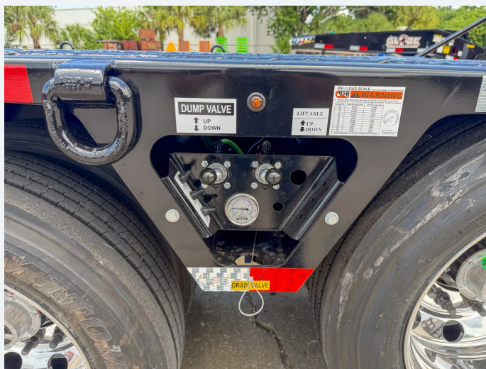
Clearly labeled air and hydraulic controls
