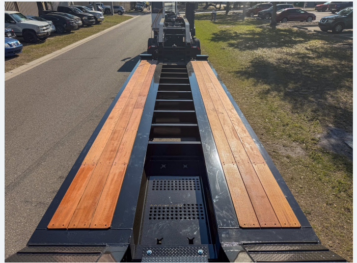
Apitong hardwood deck with recessed wells
