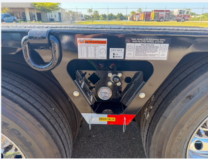
Clearly labeled air and hydraulic controls
