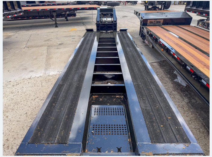
Main deck with recessed wells
