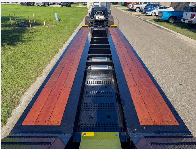
Apitong hardwood deck with recessed wells
