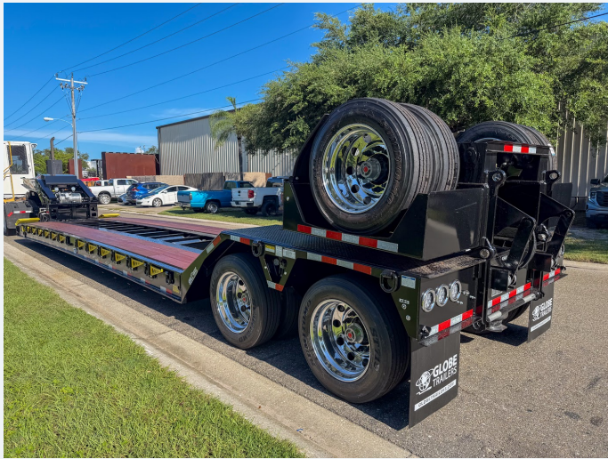
Hydraulic flip axle folds up for transport
