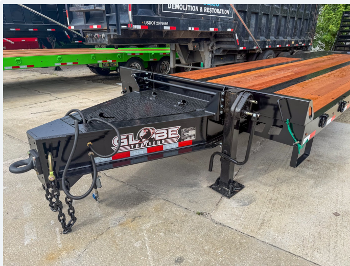
Tag-along tongue with heavy-duty jack
