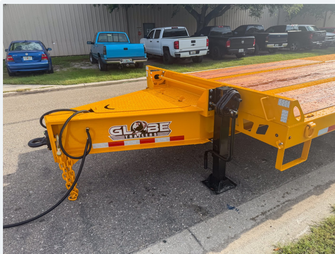
Tag-along tongue with heavy-duty jack
