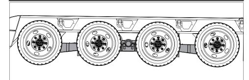
A suspension is provided that comprises a tandem axle walking beam with a vertically compliant center pivot bushing and a spring medium located over each axle center. The walking beam is rigidly attached to the axles and is pivotally coupled to a frame of the vehicle at a location intermediate of the first and second axles.
