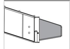
Frame has an integrated bumper with push block that's protects rear of trailer when in contact with a push machines.
