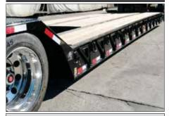
With a standard deck height of 22", Globe Trailers have lower overall height, which allows taller loads to be hauled.
