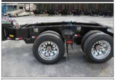
The Stinger Assembly increases the wheel base of the trailer when attached to the rear trailer frame. The Stinger Assembly is used for heavy hauling situations where regulations and specific axle loads must be adhered to.
