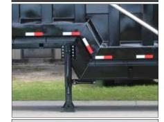
The drop deck allows for more volume and reduces overall height, also the trailer is safer than other trailers due to the lower center of gravity.
