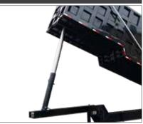
The hydraulic lift cylinder allows and restricts the trailer dumping angle up to 45°, which is optimal for ejecting debris and maintaining a safe operating height.
