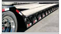
With a standard deck height of 24", Globe Trailers have lower overall height, which allows taller loads to be hauled.
