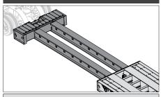
The extendable deck allows for increasing the deck length to accommodate various load lengths.
