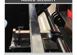
Globe Trailers air lock with safety bar and spring extended pin ensures that the gooseneck locking pin will remain secured even if air pressure is lost.
