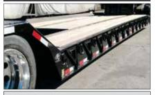
With a standard deck height of 20", Globe Trailers have lower overall height, which allows taller loads to be hauled.
