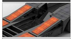
The Air Transition Ramps are recessed in the trailer deck and can quickly be activated to allow loading onto the upper deck.
