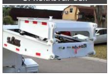
Flip box length options are available to achieve longer swing clearances when needed for longer truck frames or when coupling to single or multiaxle jeeps.
