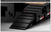
Standard Steel Front ramps, for ease of front loading.
