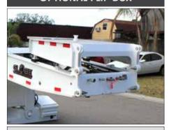
Flip box length options are available to achieve longer swing clearances when needed for longer truck frames or when coupling to single or multi-axle jeeps.
