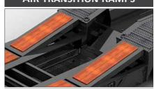
The Air Transition Ramps are recessed in the trailer deck and can quickly be activated to allow loading onto the upper deck.
