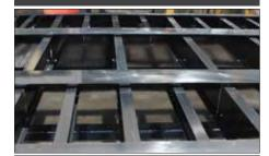
Standard 12" stubbed cross member spacing produces added strength to the trailer and also less stress on the decking, leading to a longer life of the decking material.
