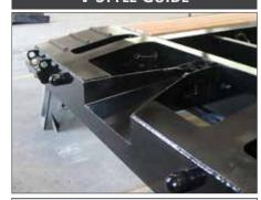
V-Style guide with front tapered beams helps position the gooseneck locking pin, which makes hooking up to a Globe Trailer fast and easy. The locking pin guide rim helps prevent the gooseneck locking pin from coming loose in transit.
