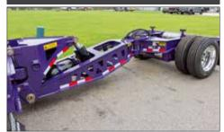
The Stinger Assembly increases the wheel base of the trailer when attached to the rear trailer frame. The Stinger Assembly is used for heavy hauling situations where regulations and specific axle loads must be adhered.
