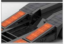
The Air Transition Ramps are recessed in the trailer deck and can quickly be activated to allow loading onto the upper deck.
