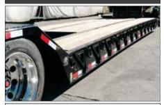
With a standard deck height of 18", Globe Trailers have lower overall height, which allows taller loads to be hauled.
