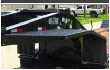
The fenders are in place to help protect the load from flying debris that a truck may create.
