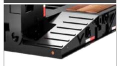
Low profile built-in integrated deck ramps.
