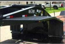
The fenders are in place to help protect the load from flying debris that a truck may create.
