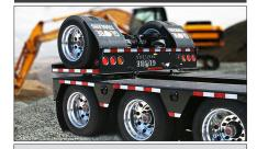
Globe Trailers has a patent on the hydraulic flip axle design. It allows for less down time when operating the flip axle and it can be easily detached when required.
