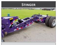
The Stinger Assembly increases the wheel base of the trailer when attached to the rear trailer frame. The Stinger Assembly is used for heavy hauling situations where regulations and specific axle loads must be adhered.
