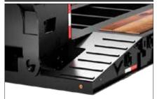
Low profile built-in integrated deck ramps.
