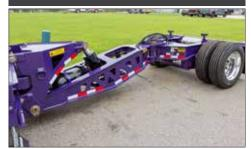
The Stinger Assembly increases the wheel base of the trailer when attached to the rear trailer frame. The Stinger Assembly is used for heavy hauling situations where regulations and specific axle loads must be adhered.
