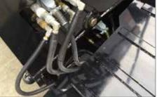
Air, electric and hydraulic (when applicable) fittings are all centrally located at the base of the gooseneck inside a bolster. This makes for quick and easy connect and disconnect. The fittings are protected from possible contact with equipment being loaded or unloaded.
