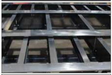
Standard 12" stubbed cross member spacing produces added strength to the trailer and also less stress on the decking, leading to a longer life of the decking material.
