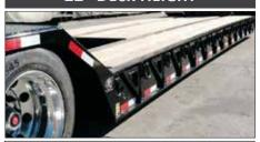
With a standard deck height of 22", Globe Trailers have lower overall height, which allows taller loads to be hauled.
