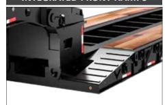
Low profile built-in integrated deck ramps.
