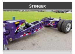
The Stinger Assembly increases the wheel base of the trailer when attached to the rear trailer frame. The Stinger Assembly is used for heavy hauling situations where regulations and specific axle loads must be adhered.
