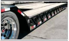
With a standard deck height of 22", Globe Trailers have lower overall height, which allows taller loads to be hauled.
