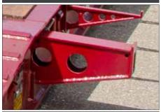
Globe Trailers fabricated heavy duty pullout front outriggers provide added strength which is needed to accommodate the initial force when loading equipment. The outrigger is held in position with a spring loaded locking pin.
