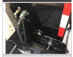
Air, electric and hydraulic (when applicable) fittings are all centrally located at the base of the gooseneck inside a bolster. This makes for quick and easy connect and disconnect. The fittings are protected from possible contact with equipment being loaded or unloaded.
