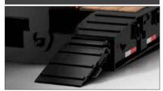
Standard Steel Front ramps, for ease of front loading.
