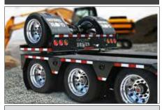
Globe Trailers has a patent on the hydraulic flip axle design. It allows for less down time when operating the flip axle and it can be easily detached when required.
