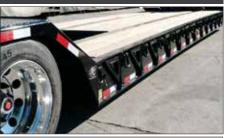
With a standard deck height of 24", Globe Trailers have lower overall height, which allows taller loads to be hauled.
