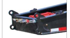
Flip box length options are available to achieve longer swing clearances when needed for longer truck frames or when coupling to single or multi-axle jeeps.
