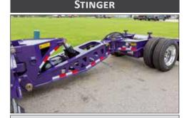
The Stinger Assembly increases the wheel base of the trailer when attached to the rear trailer frame. The Stinger Assembly is used for heavy hauling situations where regulations and specific axle loads must be adhered.
