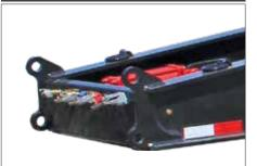
Flip box length options are available to achieve longer swing clearances when needed for longer truck frames or when coupling to single or multi-axle jeeps.
