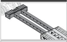
The extendable deck allows for increasing the deck length to accommodate various load lengths.
